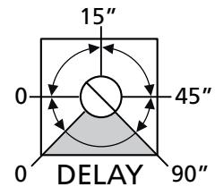
**DELAY:** time delay between the two gate leaves (0 - 90 seconds).
