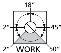
**WORK:** motor operating time (2 - 50 seconds)
